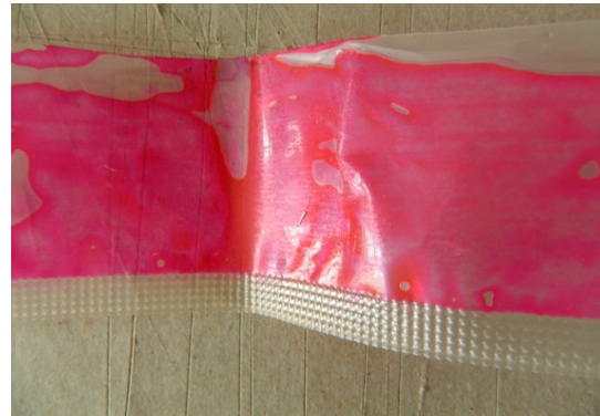
Dye penetration test for seal integrity
