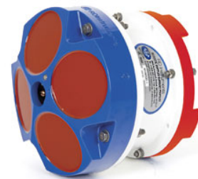
Figure 7 Core of the DREM instrument: RDI Workhorse Rio Grande (Source: RDI)
